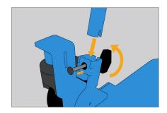
Slide the support bar down to insert into the base. The horizontal bar and the hooks must be on the same side as the handle on the
